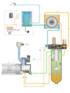
Intake air Air/oil mixture Wet compressed air Condensate
